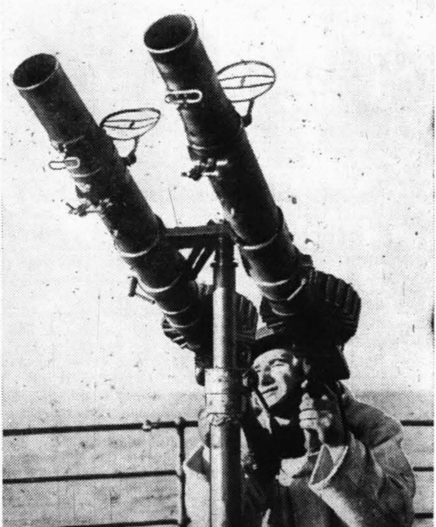
With a British convoy. The various types of gun used by the British Navy are proving very effective against the menace of German U-boat and air attack on British convoys. An expert naval gunner sighting a twin Lewis gun on board one of the protecting vessels of the convoy.
